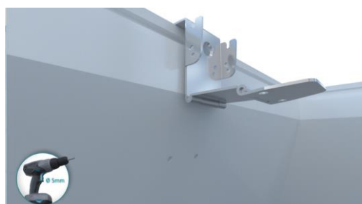
6. Löcher bohren (5mm) Drill holes (5mm)
