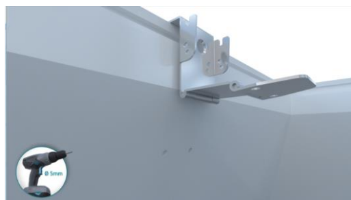
6. Löcher bohren (5mm) Drill holes (5mm)
